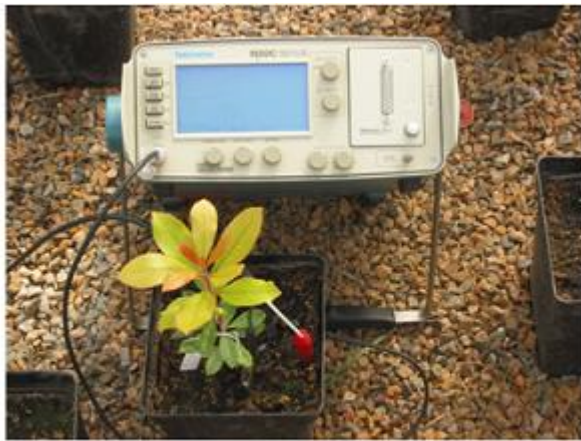
Fig. 2. Monitoring Arbutus unedo plants using Time Domain Reflectometry (TDR)
